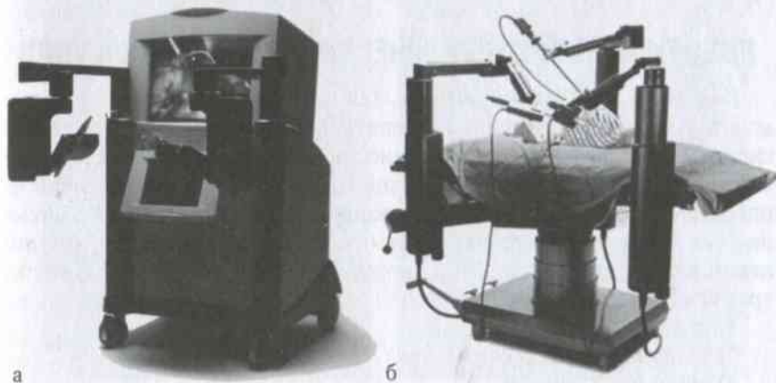
Рис. 16-13. Роботическая хирургическая система ZEUS (Computer Motion): а — подсистема хирурга; б — подсистема пациента. [Damiano R.J. et al. Initial United States clinical trial of robotically assisted endoscopic coronary artery bypass grafting // The Journal of Thoracic and Cardiovascular Surgery. — 2000, Jan. — Vol. 119. — Issue 1. — P. 77-82]
