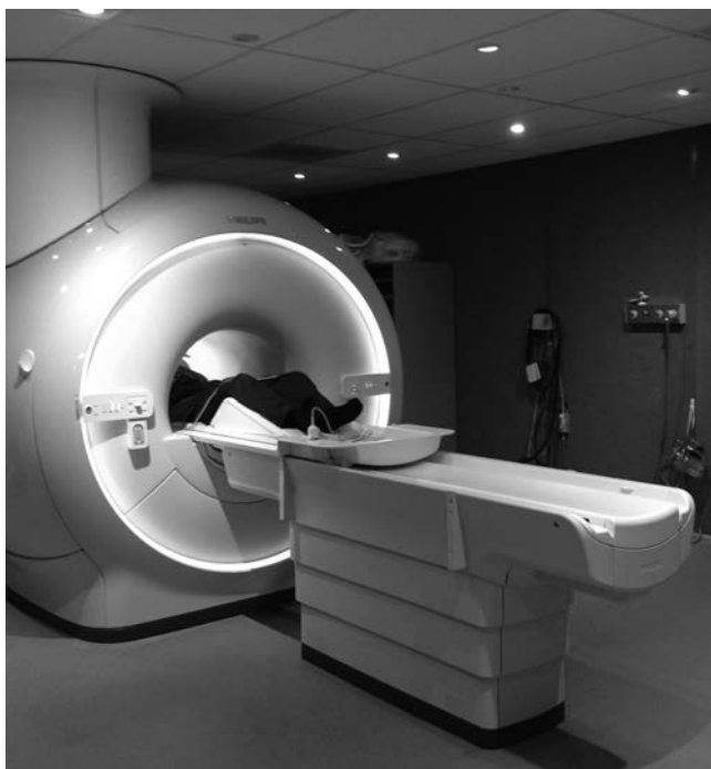
FIG. 23.3.1 Typical 3-Tesla short bore, 70-cm opening diameter magnetic resonance imaging machine.
