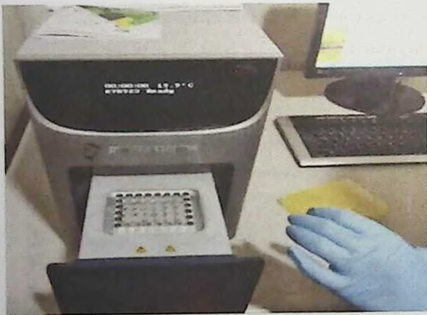
Rice. 2.5. Installing test tubes in the block of the detecting cycler
