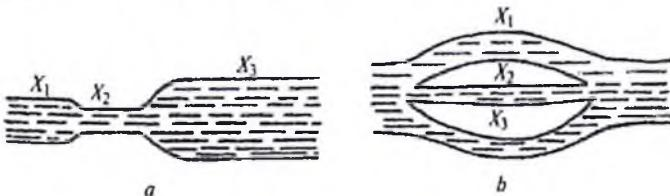
**3.6-Rasm.** Ketma ket (a) va parallel (b) ulangan trubalarda suyuqlikning harakati
