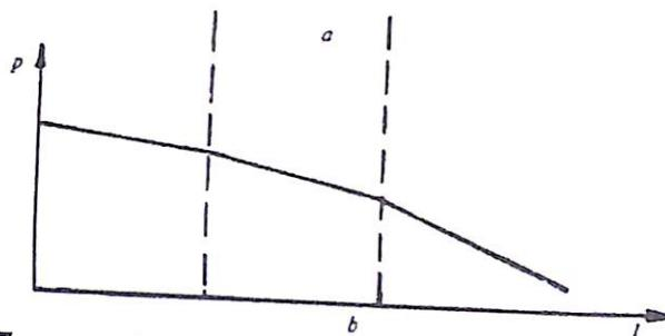
**3.7-rasm.** Suyqulikning truba bo'ylab harakati.
