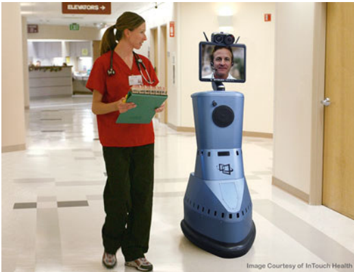
Fig. 18.5 Telehealth robot. This is controlled by a remote clinician, and includes videoconferencing and remote monitoring capabilities. In this example, physician is speaking with a nurse while conducting remote patient rounds (Source: InTouch Health, reproduced with permission)
