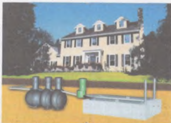
17-rasm. Suyuq chiqindilarni tozalash uchun mahalliy inshoot sxemasi
