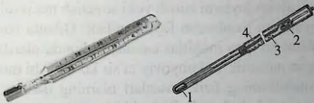
4.12-rasm. a-simobli termometr, b-metastatik termometr: 1-rezurvar, 2-qo'shimcha kamera, 3-kamera, 4-asosiy shkala
