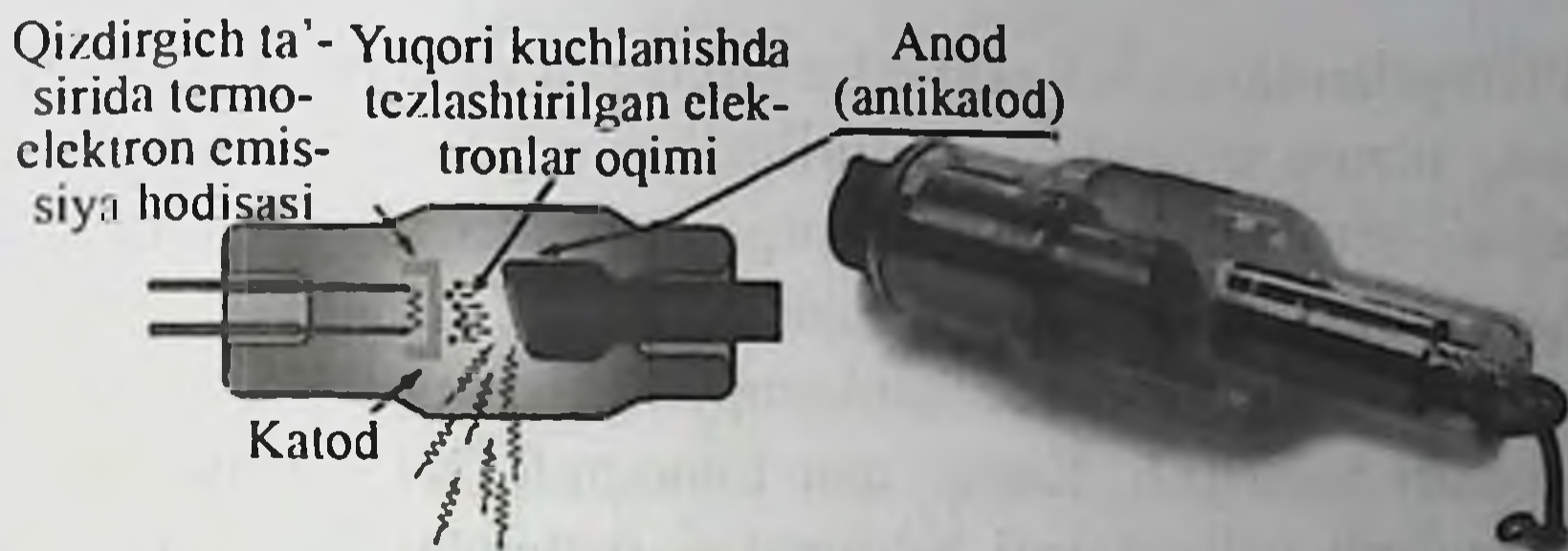
8.6-rasm. Rentgen trubkasining tuzilishi.
