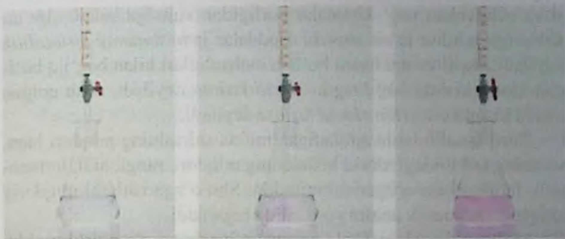
12.5-rasm. Tekshirilayotgan HCl ning miqdorini NaOHning ishchi eritmasi bilan titrlash. Indikator fenolftalien
