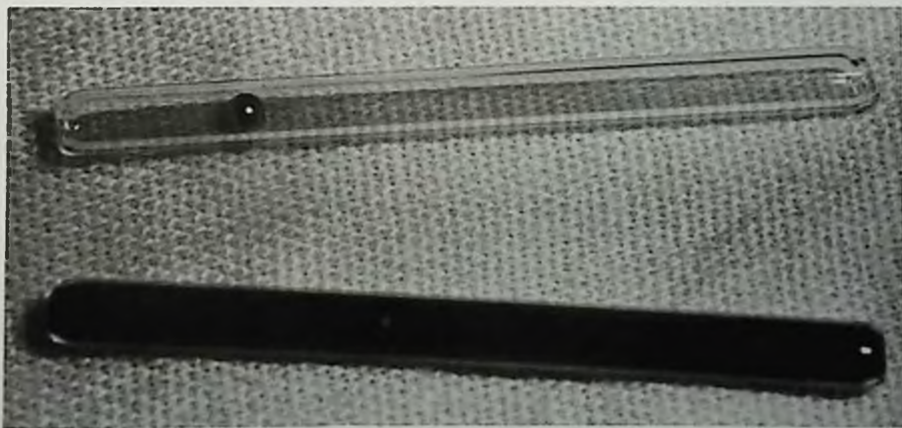
Fig 1-3. —Laidlaw clotting time tubes. Note metal ball in both empty and blood-filled tubes. (Courtesy of McDonald, M. M., and Hathaway, W. E.: J. Pediatr. 101:451-457, September 1982.)
