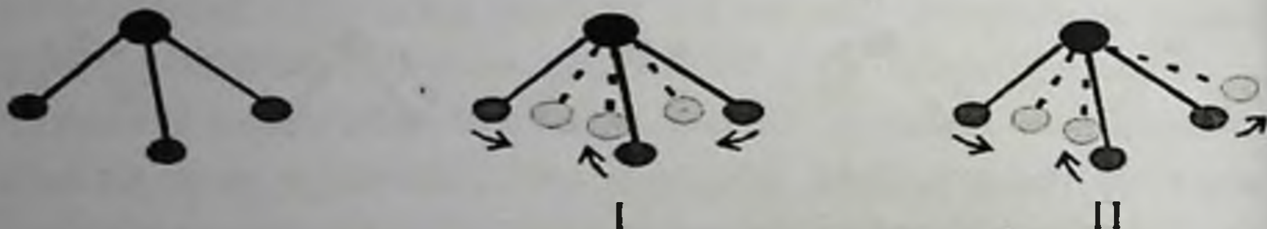
2.14-rasm. Metil guruhining simmetrik (I- 1380 \text{ sm}^{-1} ) va asimmetrik (II- 1460 \text{ sm}^{-1} ) deformatsion tebranishlari.
